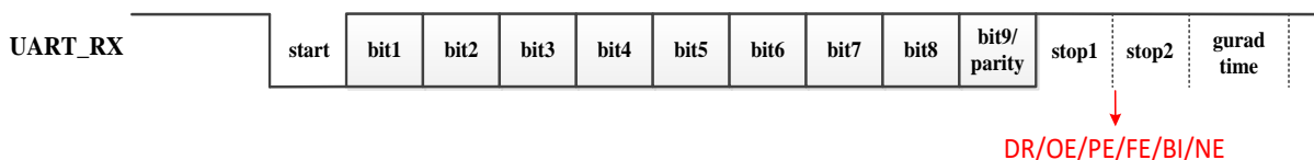
Figure 9-3 UART receiver flow
